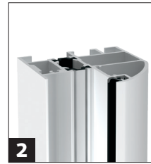
2 60mm aluminium frame (FrontGuard 46) or 80mm aluminium frame (FrontGuard 65). Both with built in thermal break.
