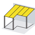
Pent roof with roof guttering offset
