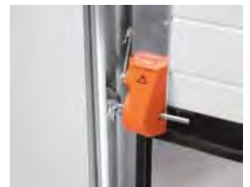
Cable break device that engages in the event of cable breakage that instantly stops the door from closing (optional).
