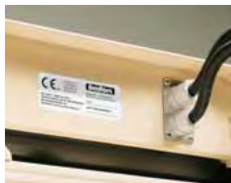
CE marking product identification data plate stating all the data required by current regulations.
