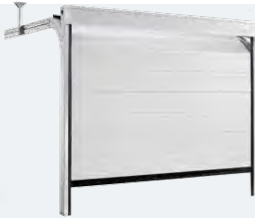
External view of Onda 250 sectional door, embossed wood finish with fixed panel shaft cover. Pre-painted similar to RAL 9010 colour and galvanized steel frame are standard. The panel interior has an embossed stucco finish in white similar to Ral 9010.
