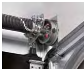
Cable break device that engages in the event of breakage of the springs that instantly stops the door from closing.
