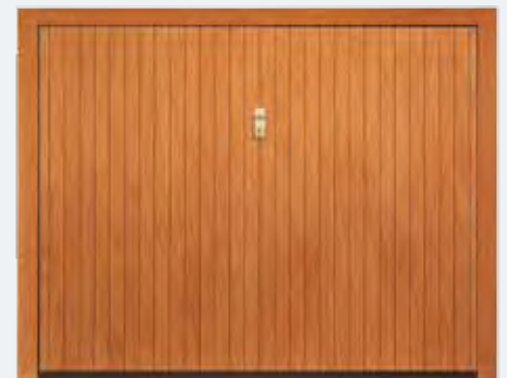
External view of Reserve Sikura HF up-and-over door, covered with multi-ply okoumé and outer cladding in oak decorated by pantograph with horizontal slats with an 85 mm pitch. The outer cladding in oak, full treatment with colour 1 and the lock with Defender art. 94 are optional.
