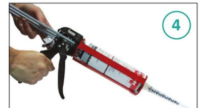
**PLEASE NOTE: ChemFix sets quickly.** Once you have applied it to the first 9-12 holes, twist the studding into each hole. Remove any excess ChemFix before it sets. Repeat this procedure until all holes are filled and leave to set for 60 minutes. Remember to change the Applicator nozzle.
